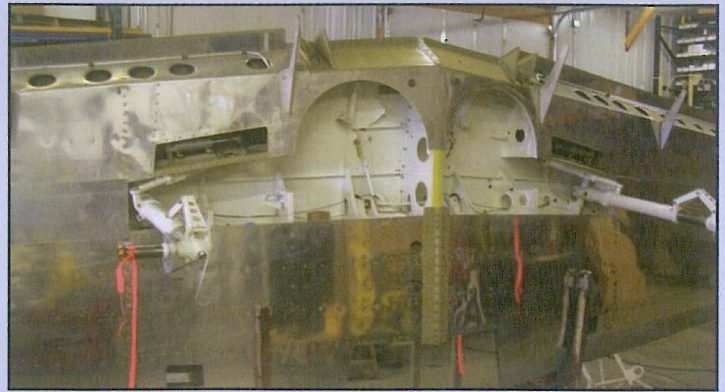
This wing was built in original factory jigs, and is ready to be mated to the fuselage.
