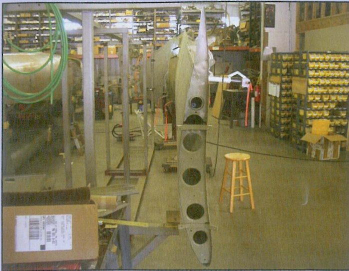
The secret of the Navion's short-field performance is in the huge wing area, the big and effective flaps, and the camber to the wing, as shown by this photo.
