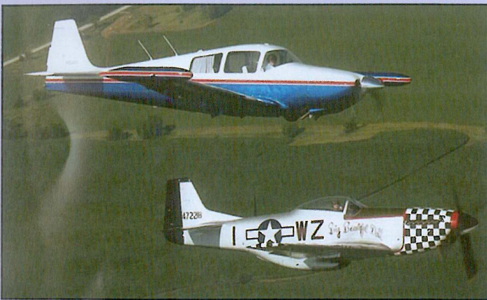
The secret of the Navion's short-field performance is in the huge wing area, the big and effective flaps, and the camber to the wing, as shown by this photo.
