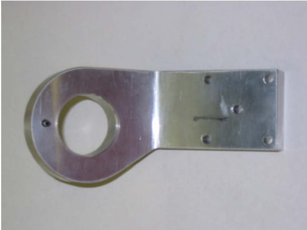
Figure 1: Sample Support with Insufficient Edge Distance
