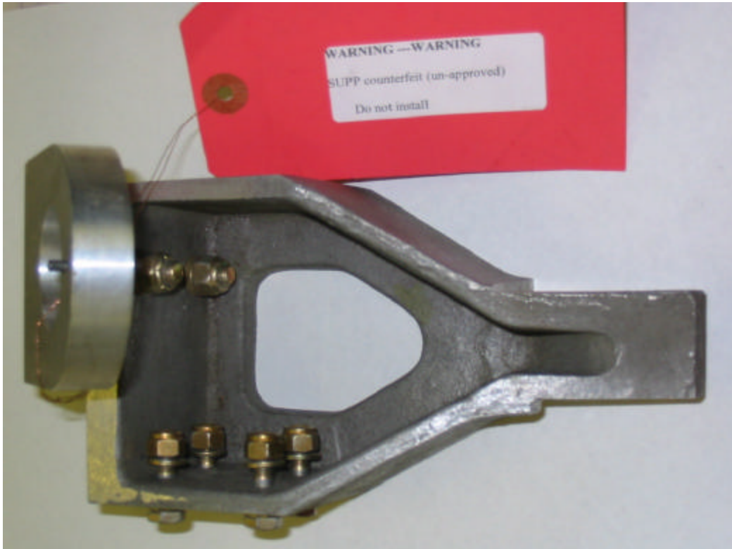
Figure 2: Casting Showing Improper Machining & Inconsistent Wall Thickness
