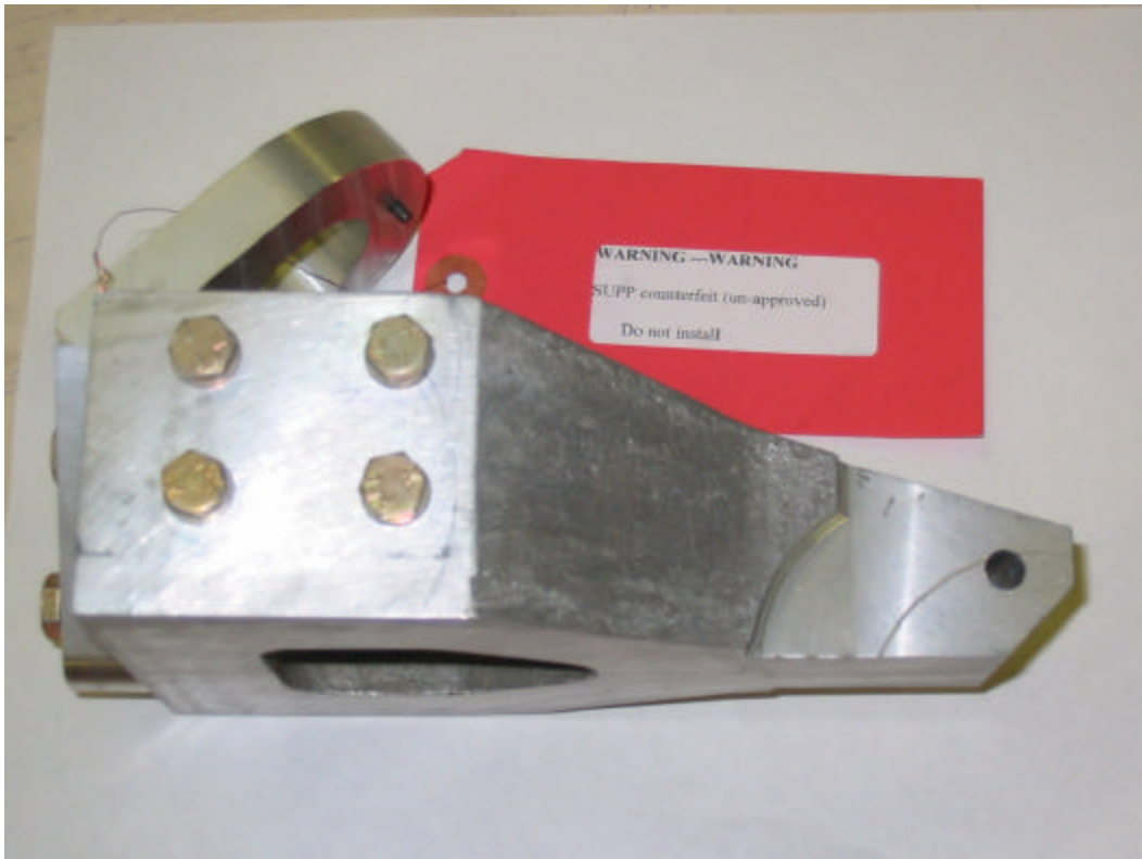
Figure 3: Casting Showing Improper Machining & Chamfer Instead of Radius
