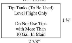
Baggage Tank Placard to be installed in accordance with Navion special instructions letter number 8. (not to scale per drawing)
