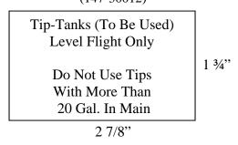
Tip-Tank Placard Sample (not to scale per drawing)
