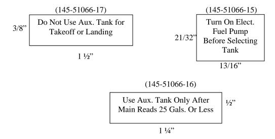
Tip-Tank Placard Sample (not to scale per drawing)
