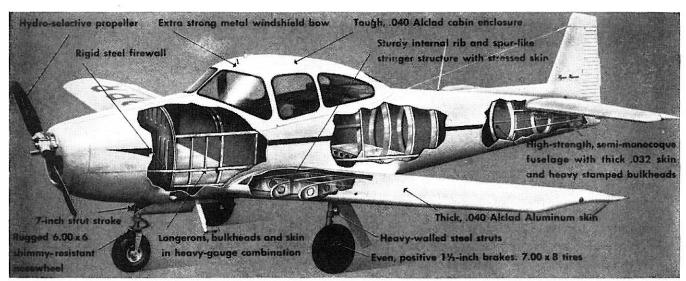
IT'S REALLY AS SIMPLE AS THIS: Navion is designed to be a safe, easy-to-fly plane. Within this fundamental premise, all other features are developed to the highest point possible. Navion is big and fast. It is rugged as a mule, and as hard-working. Aerodynamically and struc-
